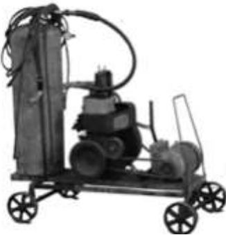
An air compressor that I made out of a Wisconsin gas engine, a 5 HP electric motor and a propane tank.
